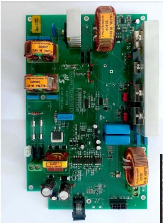
Power supply board used for Medical equipment.
